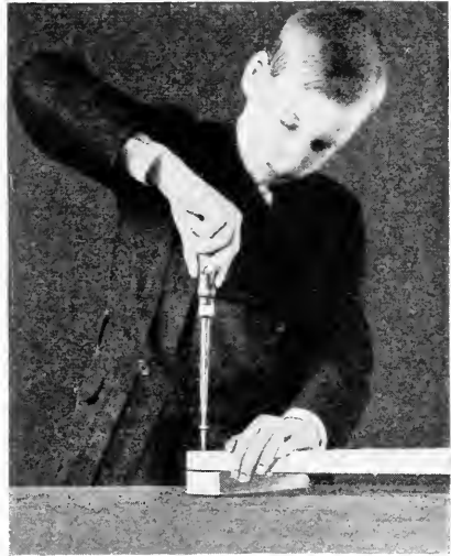
Fig. 14. Proper Position to Hold Screw Driver
